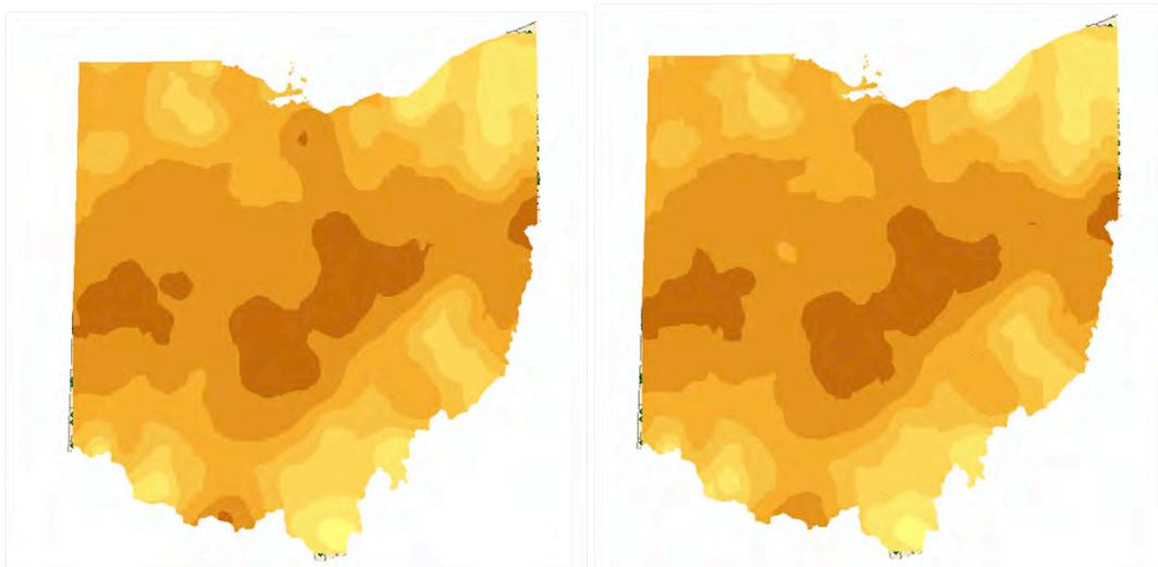
Figure 4: Spatial Distribution of Radon Concentrations in Ohio using Kriging and Cokriging Interpolation Techniques (Respectively)
