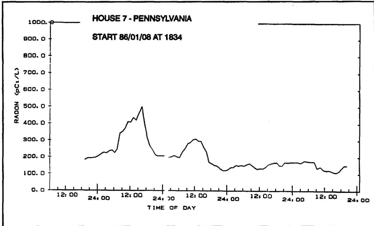
Occupant-driven diurnal changes are usually much larger than the natural cycles, as illustrated in Figure 4. This house was on a sloping site, and a garage was built into the basement. The rapid decreases in radon concentration measured in an enclosed basement workroom are associated with the garage door being open. This not only increases the basement ventilation rate, but decreases the house/soil pressure differential and hence the supply rate simultaneously.
