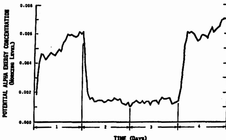
Figure 3. Reductions in PAECs provided by hassock fan-ion generator in basement room in home in Massachusetts. Fan was operated on Days 2 and 3.
