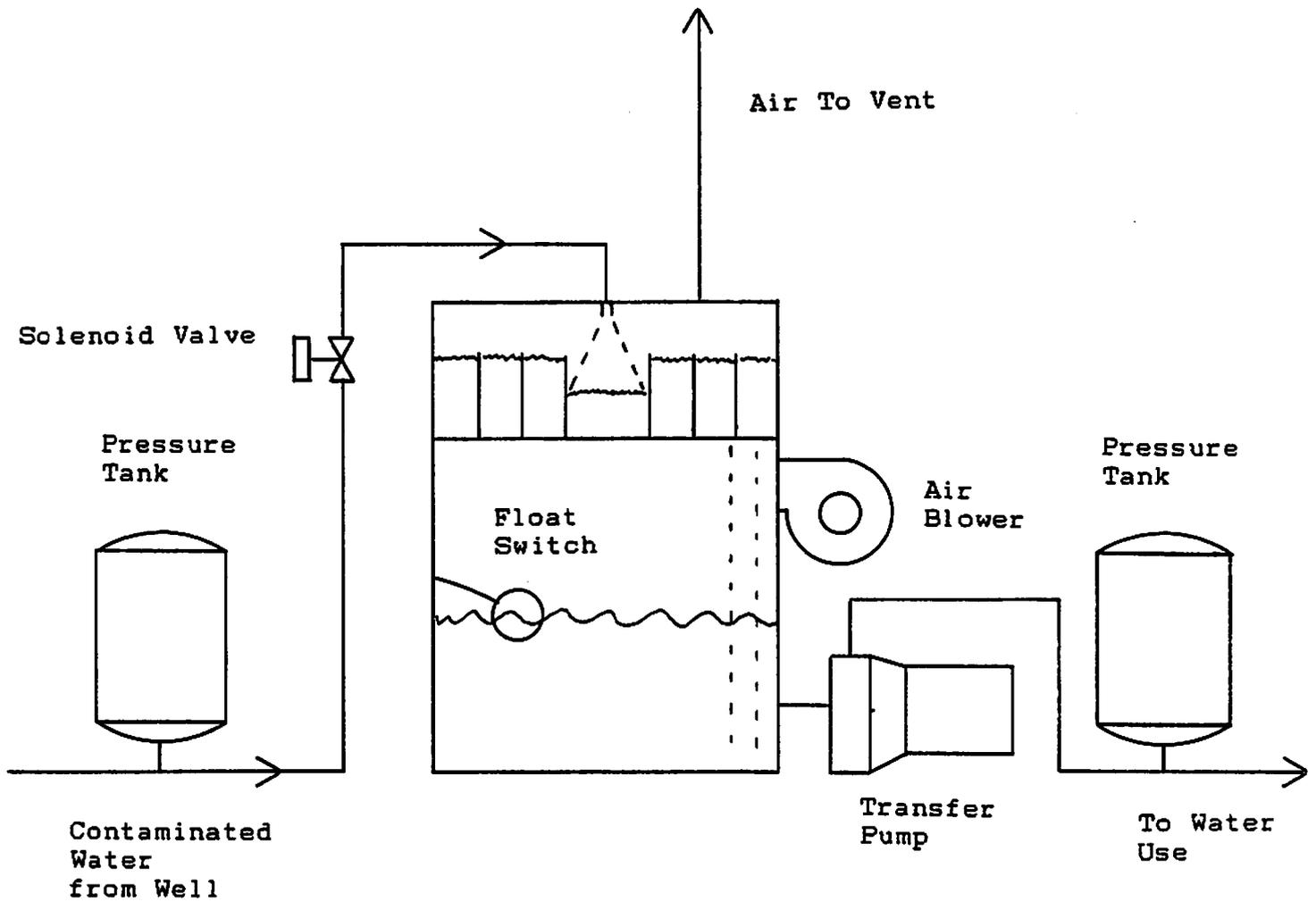
Figure 4. Horizontally Extended Shallow Aeration
