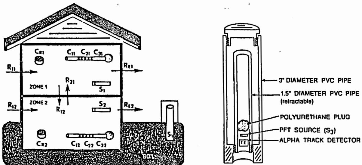
Figure 1. Schematic Representation of the Experimental System Used to Determine Multizone Radon Source Rates (after Kunz 1989)
