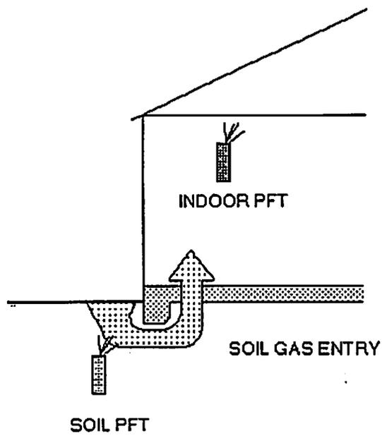
Figure 2. Schematic Representation of Deployment of PFTs to Label Soil Gas Entry in Florida Homes
