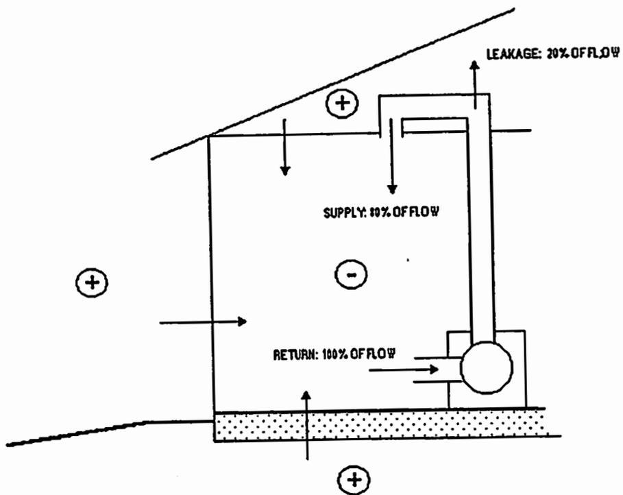
Figure 4. Depressurization of Indoor Airspace By Duct Leakage.
