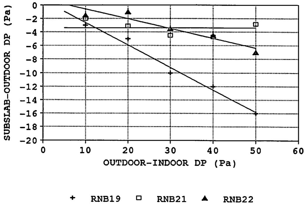
Figure 3. Depressurization of Subslab with the Blower Door.
