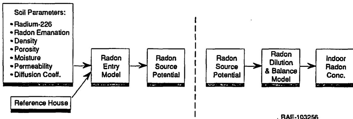
Figure 1. Partitioning of radon source and house calculations.
