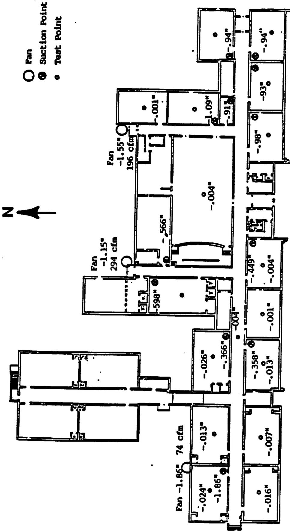
Figure 5. Post-mitigation pressure field extension, in. W. C.
