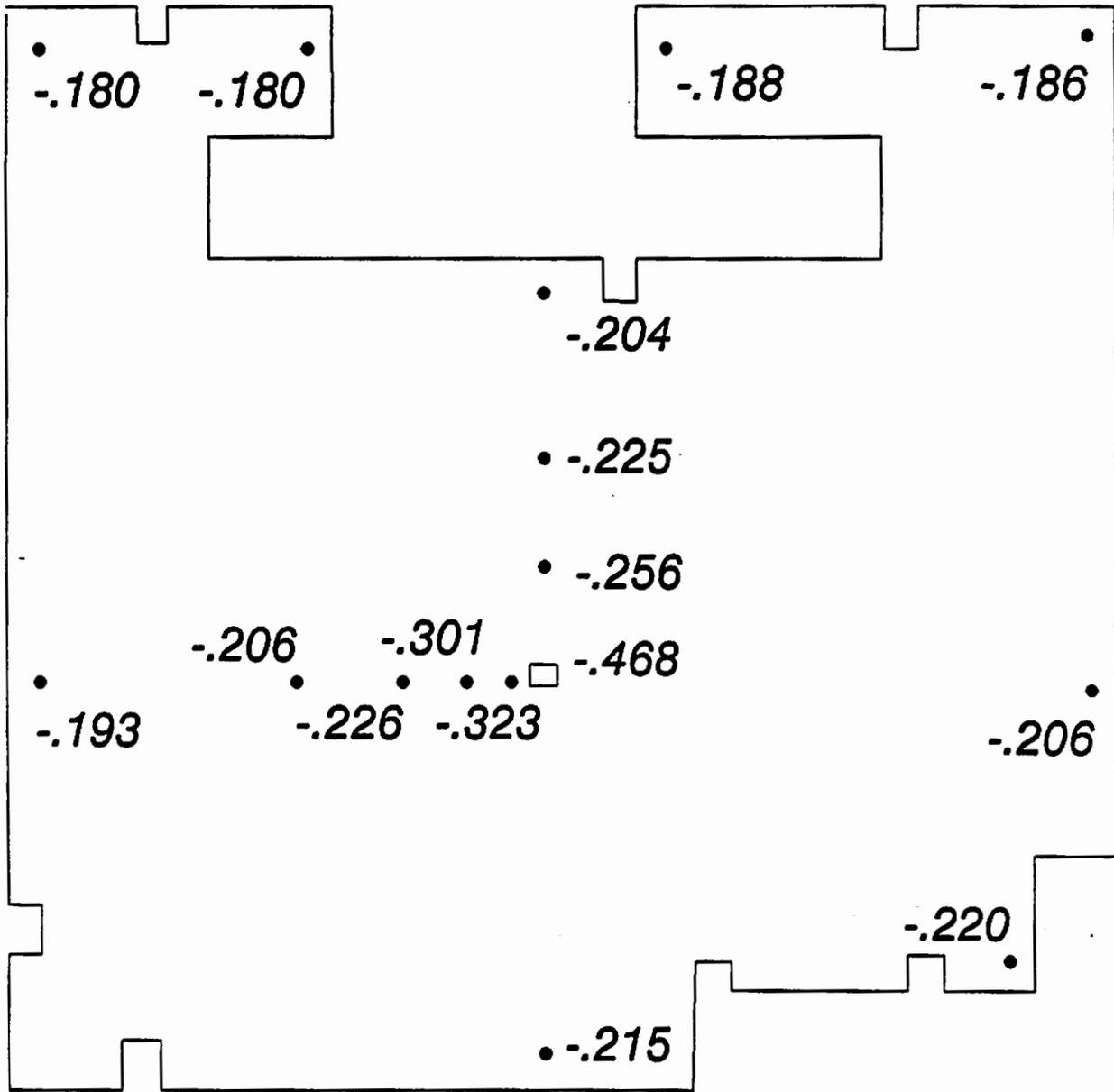
Figure 9. Subslab pressures, ASD on (in. W.C.)
