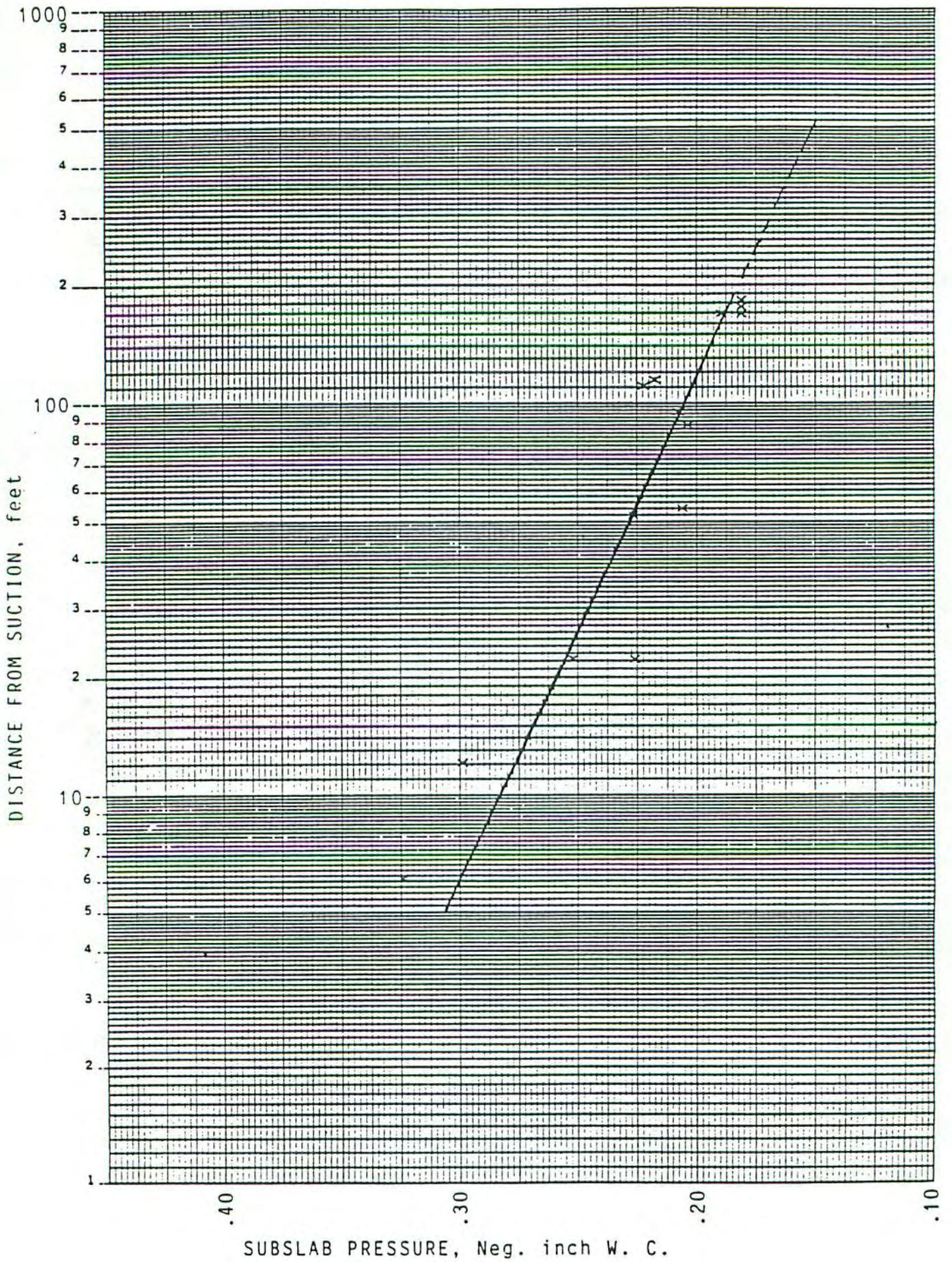
Figure 10. Pressure field extension for complete slab
