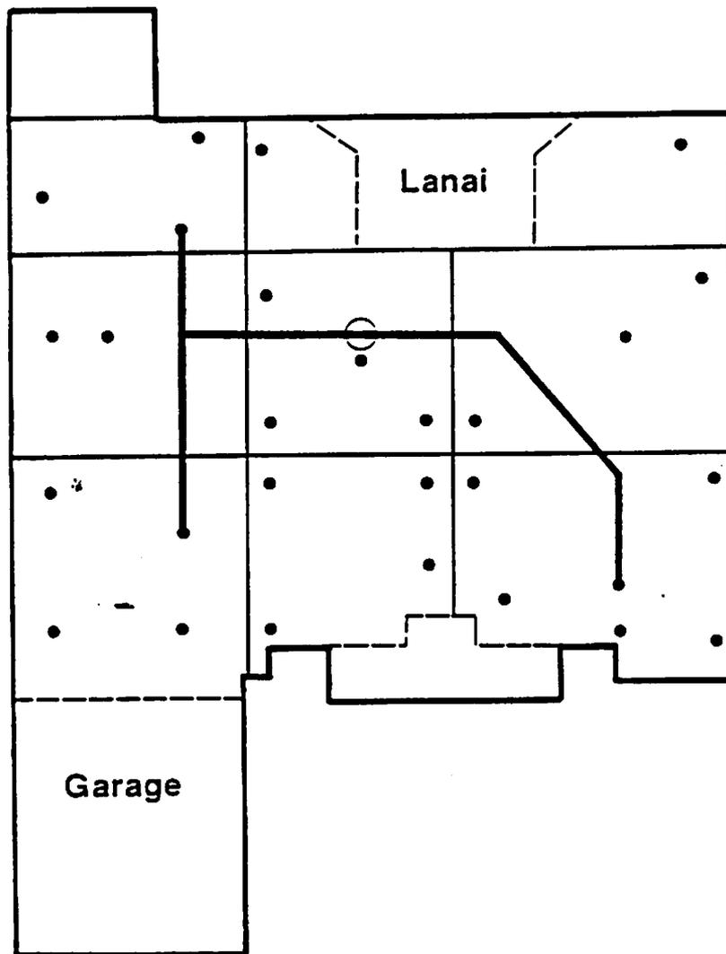
Figure 10. House #3 footprint, with mat layout, interior footer and measurement point location.
