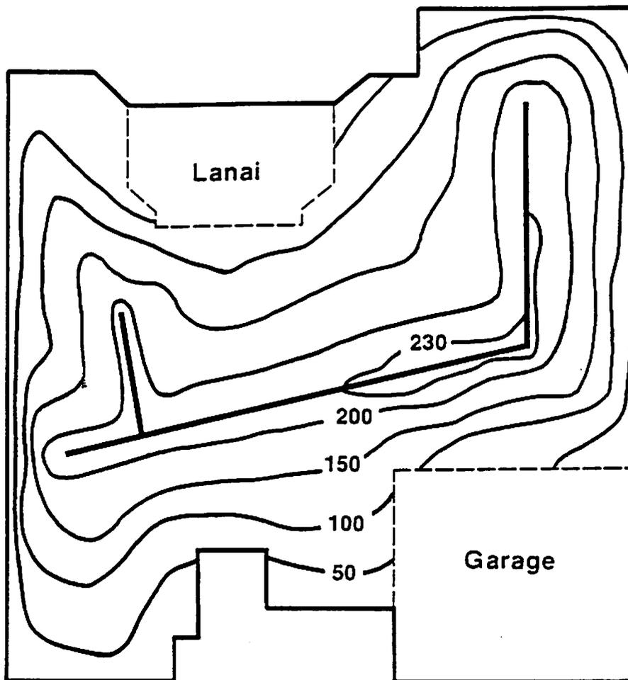
Figure 9. Presentation slide of house #4 pressure field extension.
