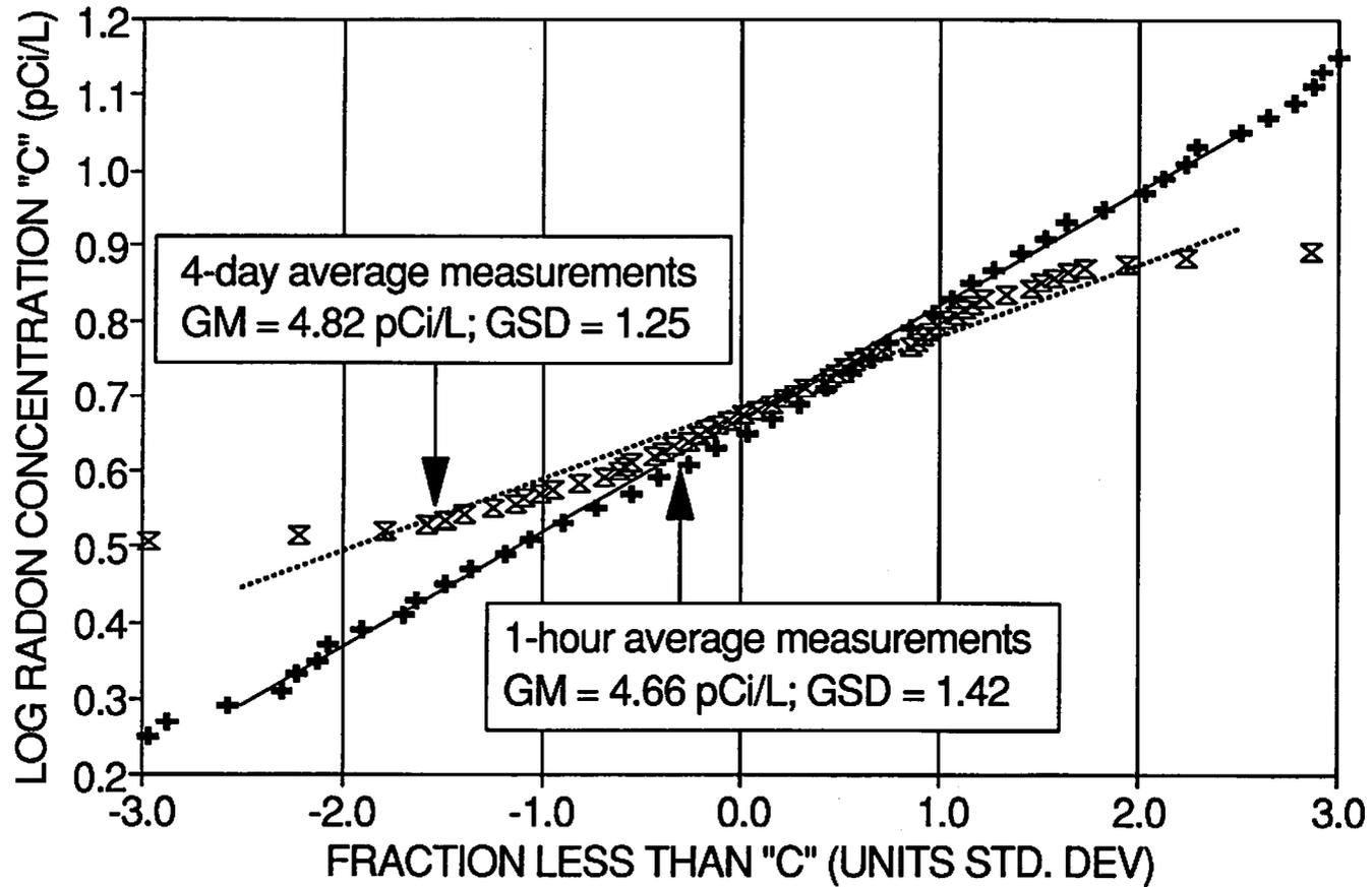
Fig 6. RADON ACCUMULATION BY CARBON FROM VARIABLE CONCENTRATION
