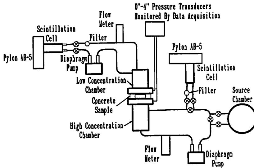
Fig. 4. Schematic of radon diffusion measurement system.
