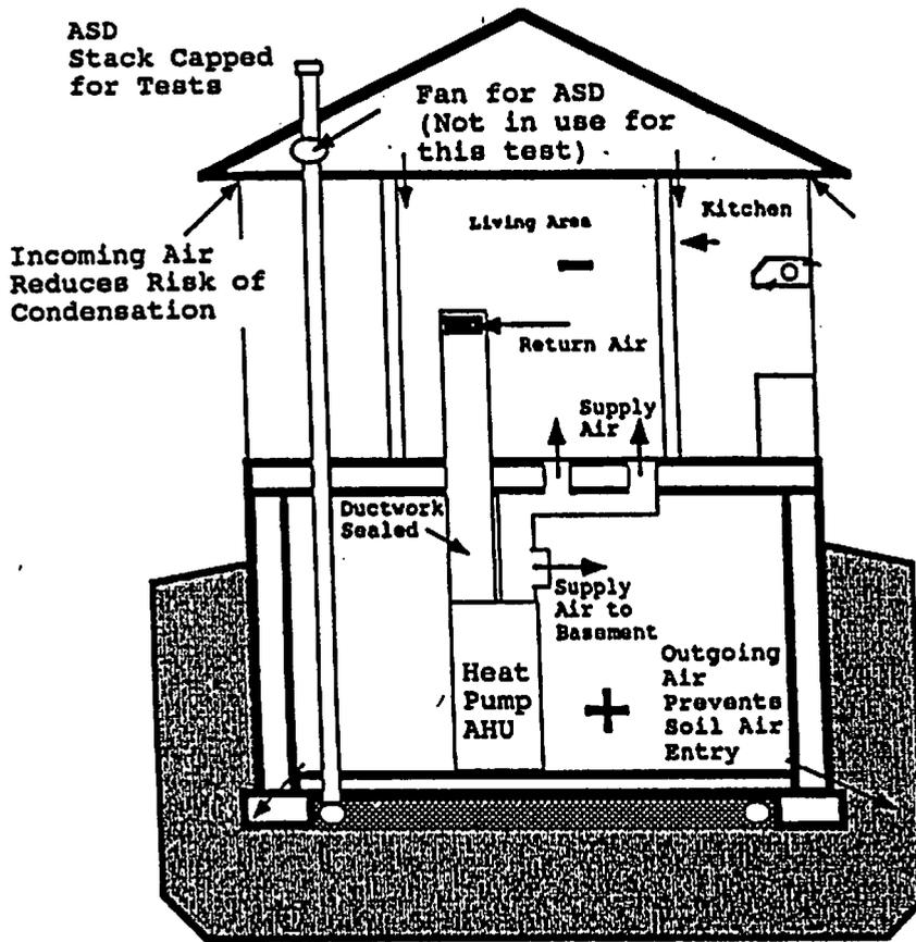
Figure 1. Showing the use of the HAC system to control radon entry, and provide recommended ventilation rates.
