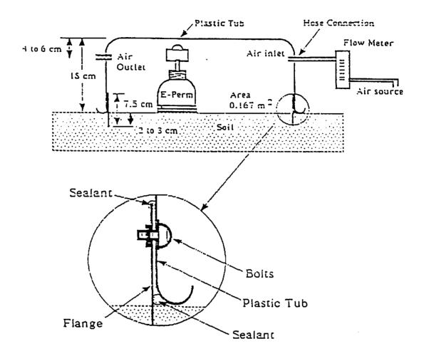
Fig. 1: The Livingston Surface Flux Monitor
