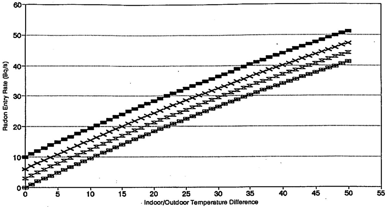
Fig. 5: Predictions of The Radon Entry Rate From The Sub-Slab Area into The Interior Generated By Temperature-Induced Pressure Differences. (Bottom to Top: No Diffusion Entry, Constant Diffusion Entries of 3, 6, & 10 Bq/s, respectively).
