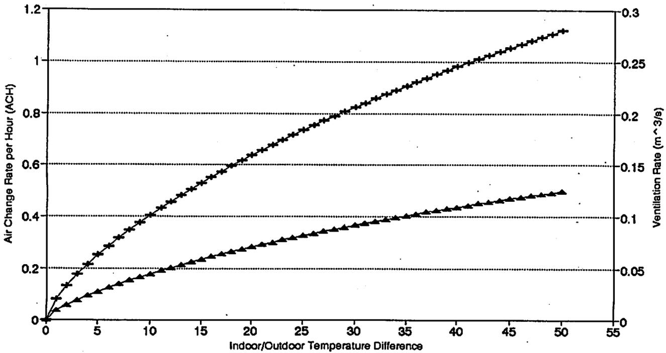
Fig. 6: The Effect of Temperature-Induced Pressure Differences on The Structure Ventilation Rates (ACH- Plus Sign).
