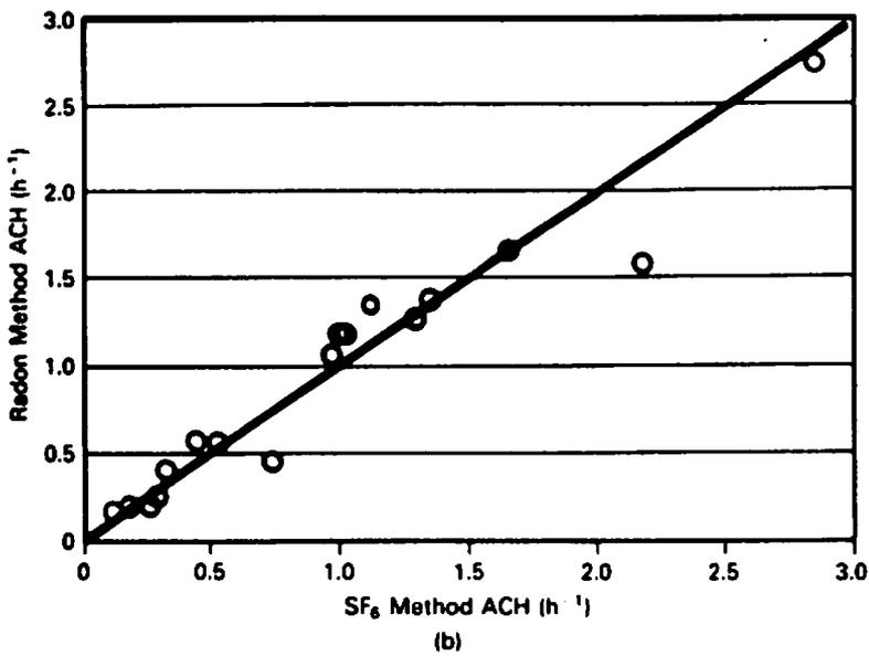
Fig. 4. Residential measured ACH values: (a) bar graph of ACH values by the SF<sub>6</sub> method (left) and the radon method (right) and (b) same data on an X-Y plot.
