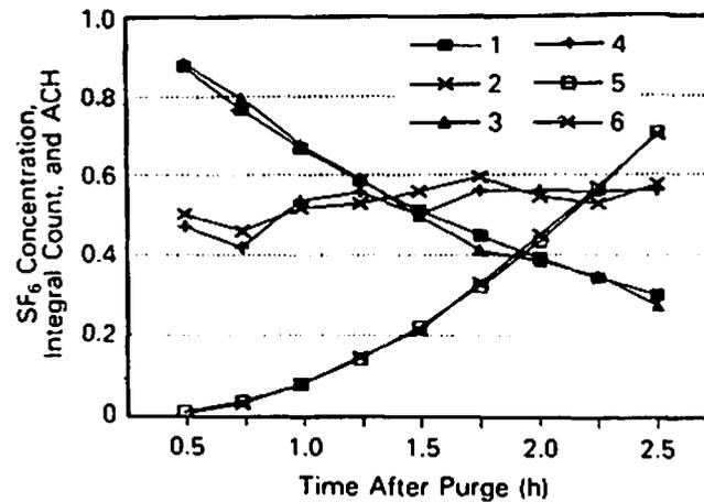
Fig. 3. Comparison of ACH time data points for the  $\text{SF}_6$  tracer gas method (curve 2) and the radon method (curve 4) for run S-2 as a function of time after purge. Also, experimental (curve 3) and theoretical (curve 1)  $\text{SF}_6$  concentration decay and experimental (curve 5) and theoretical integral count (curve 6).
