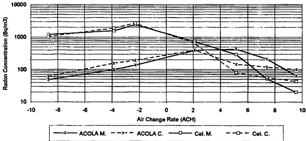
Fig 4.1 Comparison between measured results and modelling on Curves of Radon level vs. air change rate.
