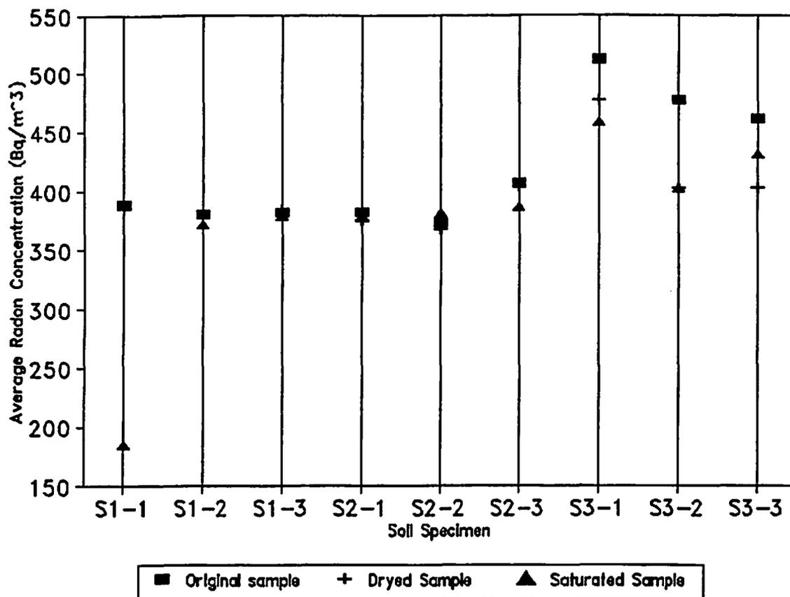
Figure 3: The response of averaged radon concentrations for original, dry, and saturated soil samples
