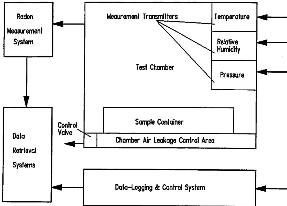
Figure 1: A Block diagram illustrating the experimental assembly used to test the effects of soil water content on in-situ soil gas radon measurements.
