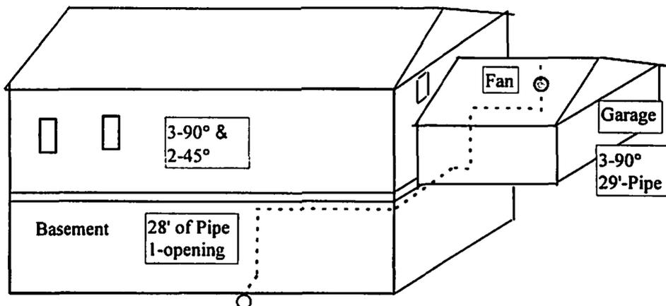
Figure 2 Example of a common ASD system with pipe routing through the garage
