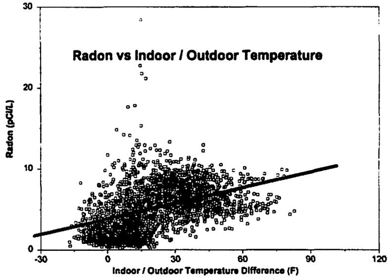
In winter when the indoor-outdoor temperature difference is maximal, the radon level can be elevated for prolonged periods of time because the house is exposed to the full impact of the stack effect.
