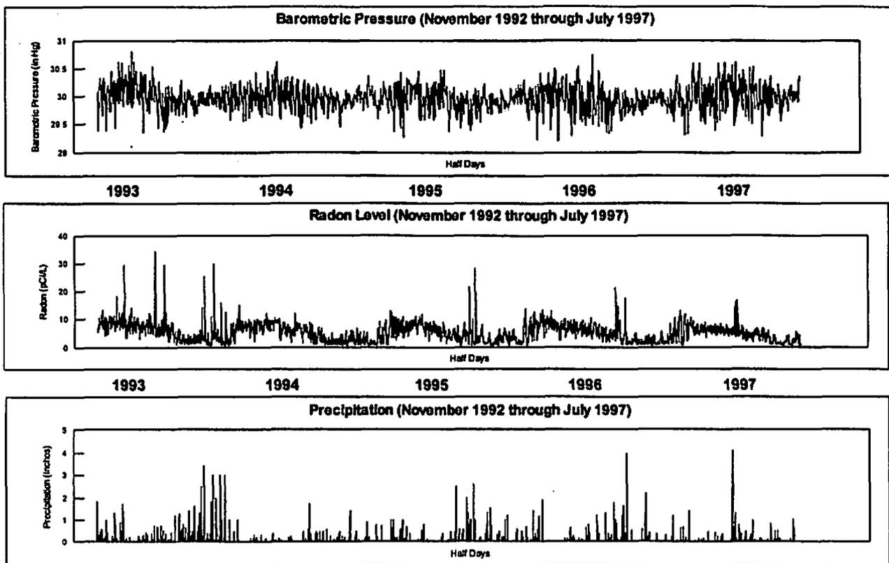
The summary graphic above illustrates the long-term impact of two major weather factors – rainfall incidents and barometric pressure changes – during the (almost) five year span of this study. Offering the long view, it illustrates the little-acknowledged impact of the weather effect on long-term seasonal variations in radon levels which might be recorded in any normally occupied home. And, too, it raises a question about the long-term validity of the long-term radon test.
