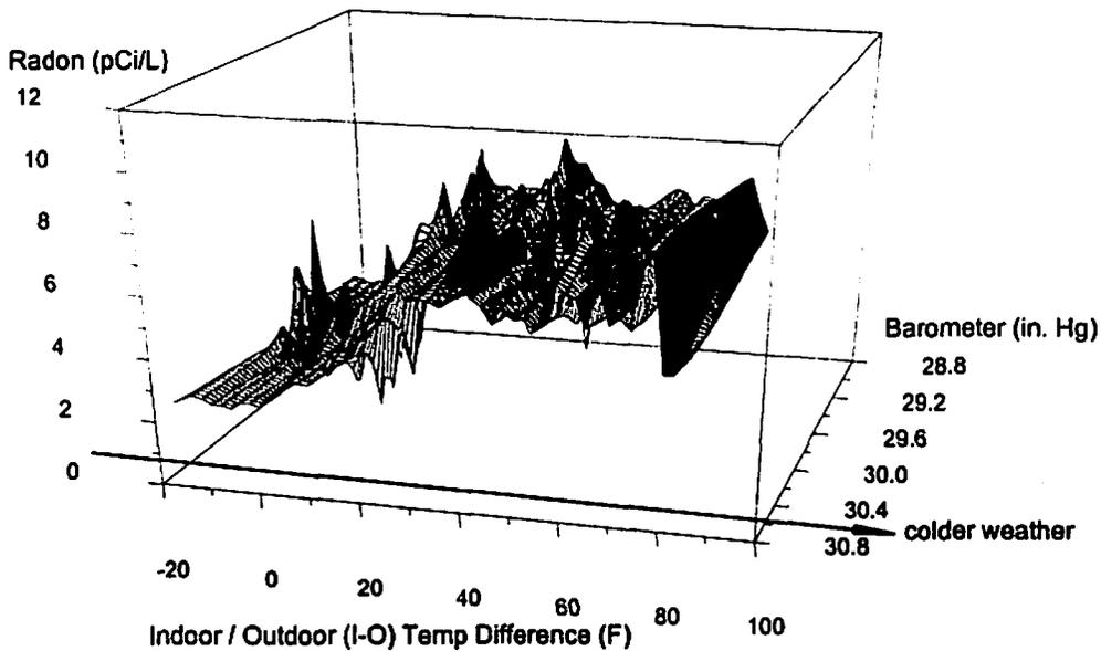
The above graphic (covering the same part of the data-set) depicts the stack effect in still another way. Note the low radon levels occurring when the temperature differences are least. Also, as indicated earlier, the more prominent radon peaks tend to be at the lower barometric pressure end of the plot.
