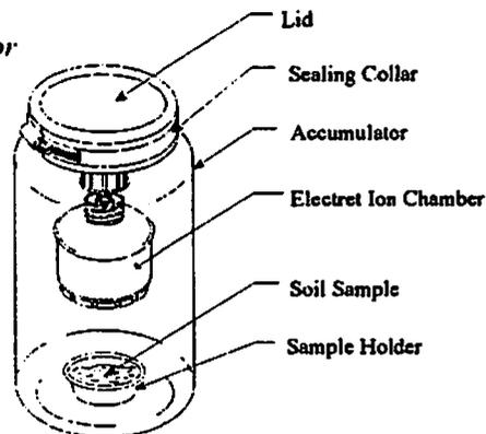
*Fig. 4-1 Radium Test Set-up*
