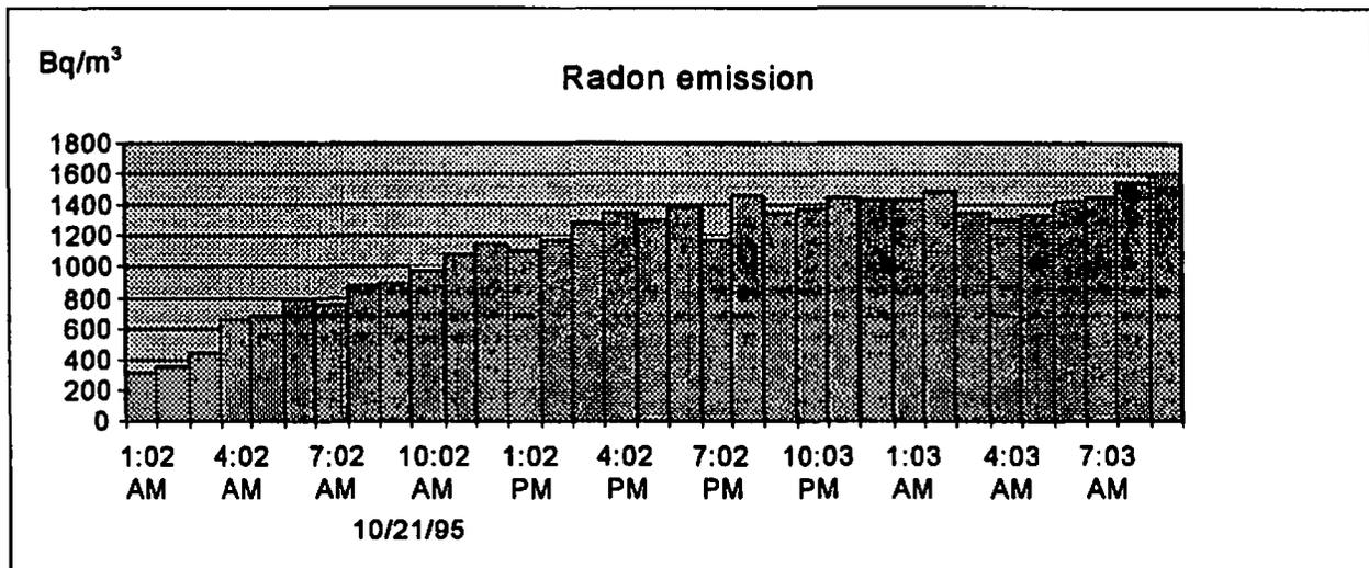
Fig 4. Measurement of radon emission from the wall.
