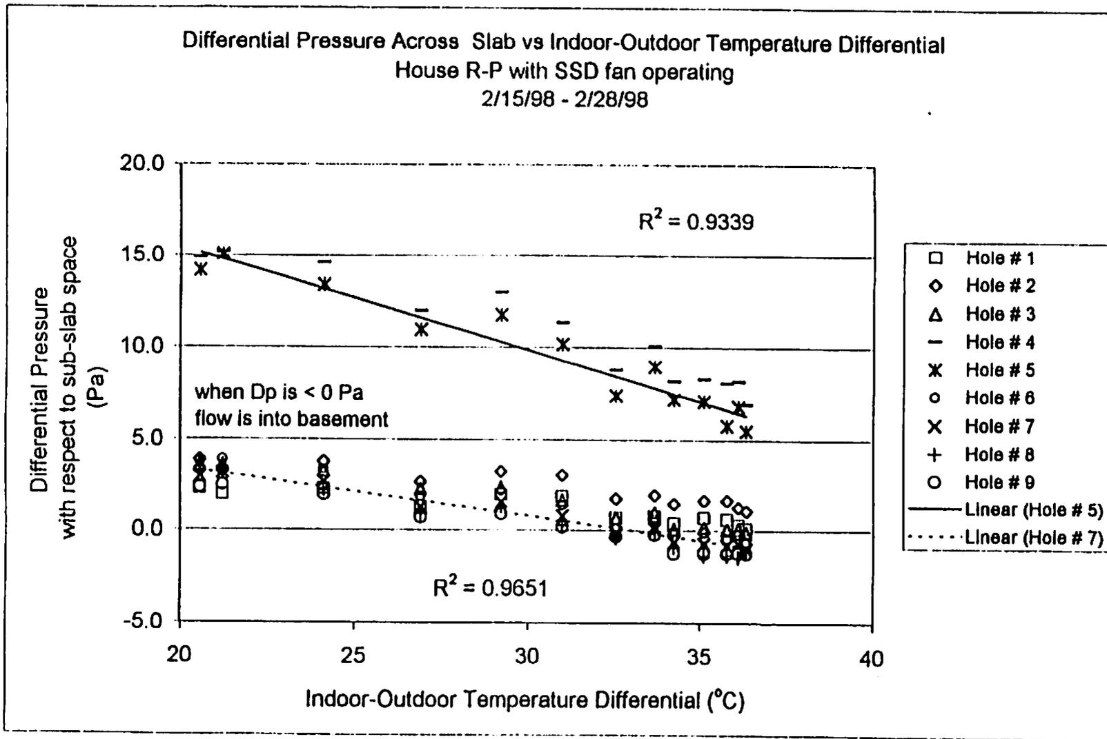
Figure 3. Dp across slab with fan on
