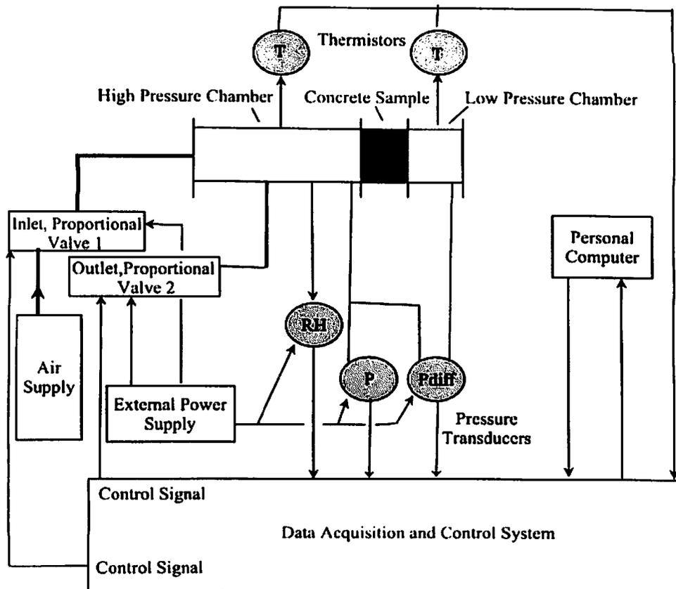
Fig. 3. Schematic diagram of system to measure the concrete sample's air permeability coefficient.
