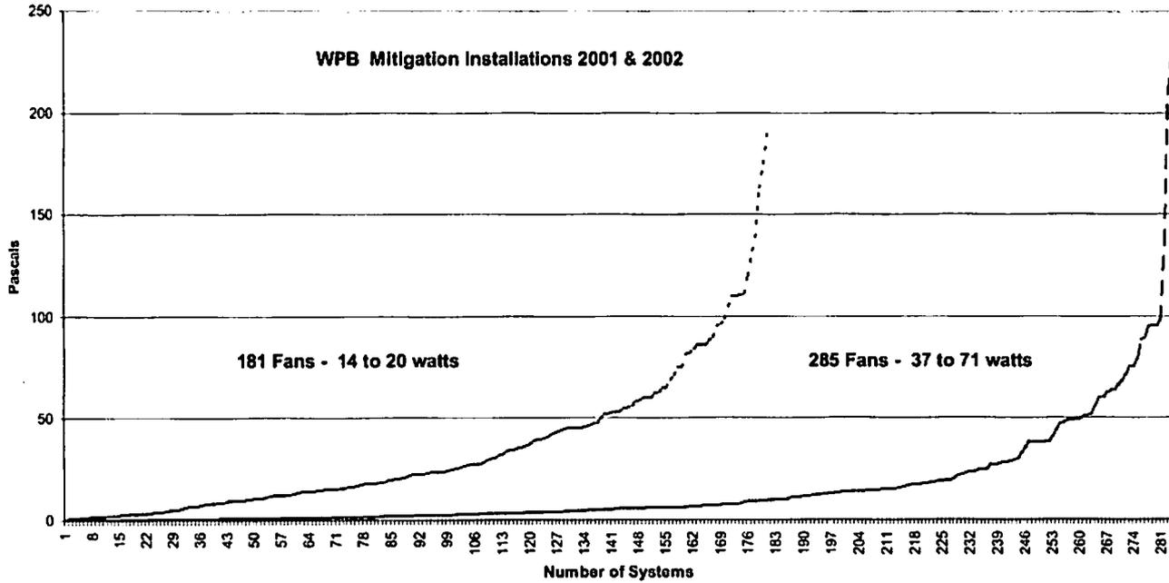
The final percentage radon reduction was actually higher for the low wattage fans than the RP145 fans. This was most likely due to use of the RP145 with more difficult buildings. Even considering this it is obvious that the low wattage fans are more than capable of reducing the radon levels in a significant number of mitigation installations.
