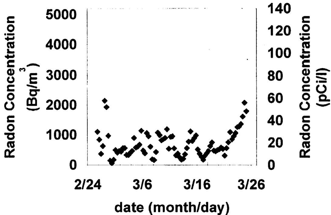
Figure 7: A plot of radon concentration versus time for the Goldstream house. During the last week of this measurement period, the ventilation system was turned off, and the result was a steady increase in radon concentration.
