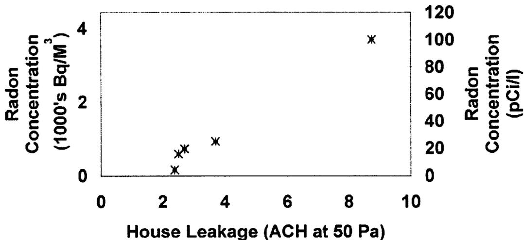
Figure 3: House air leakage versus winter radon concentration.
