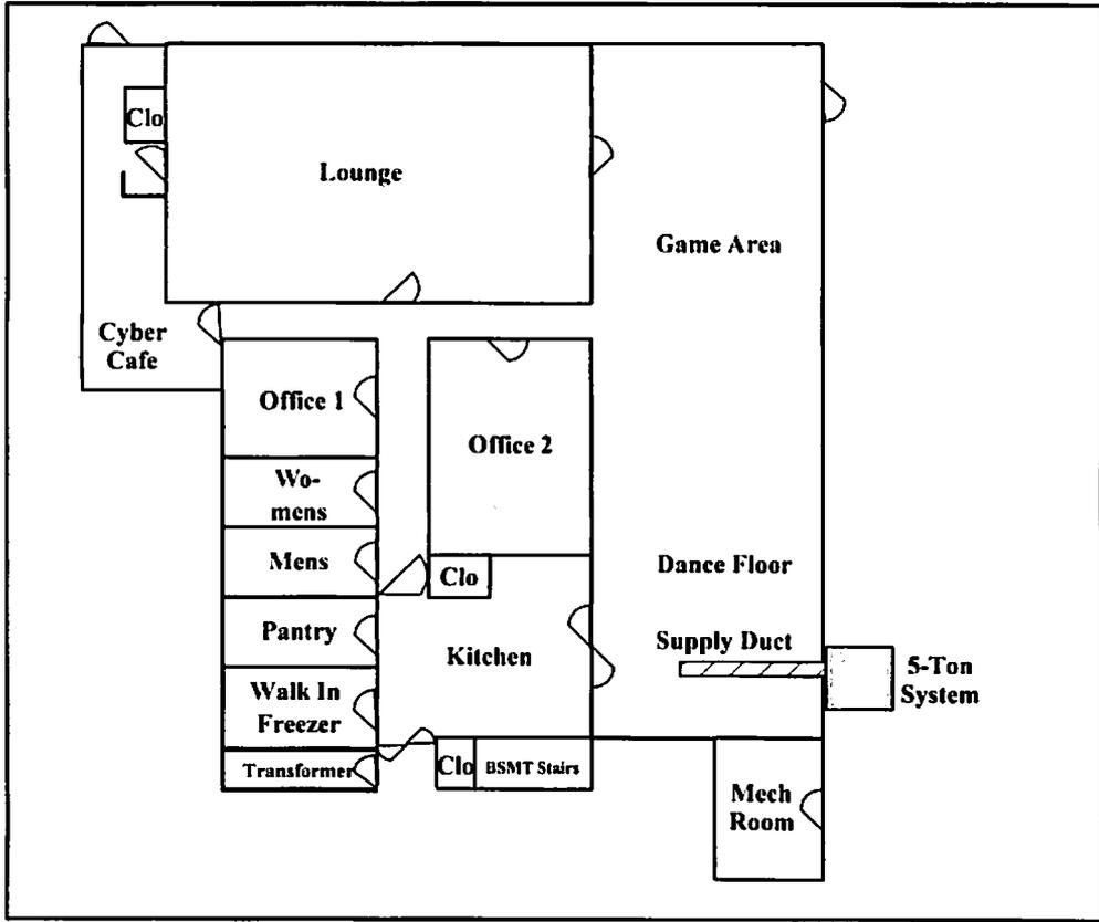
Figure 11. Location of the 5-ton supplemental air makeup system
