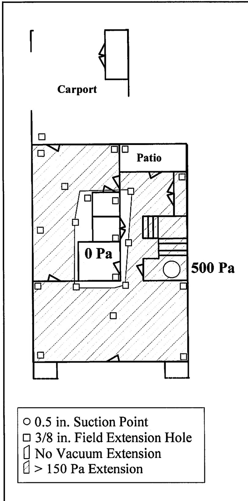
Figure 9. LFE from stairwell closet
