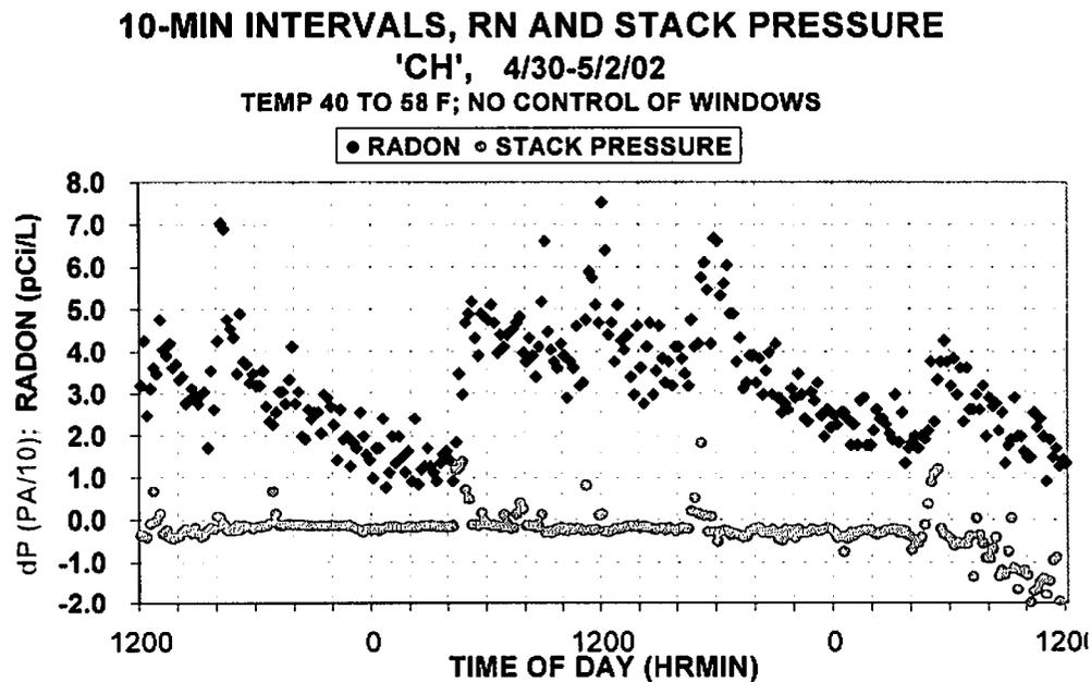
Figure 12. Radon entry at times of basement depressurization.
