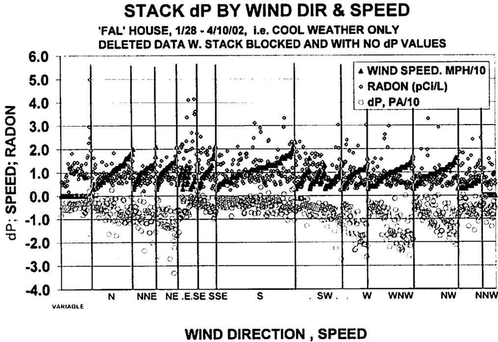
Figure 10. The effect of wind direction and wind speed on stack depressurization.
