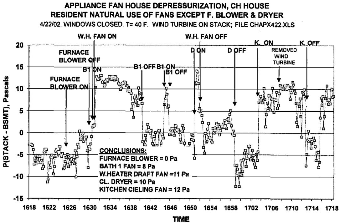
Figure 13. Pressure difference, stack base to basement, in fan depressurization tests.
