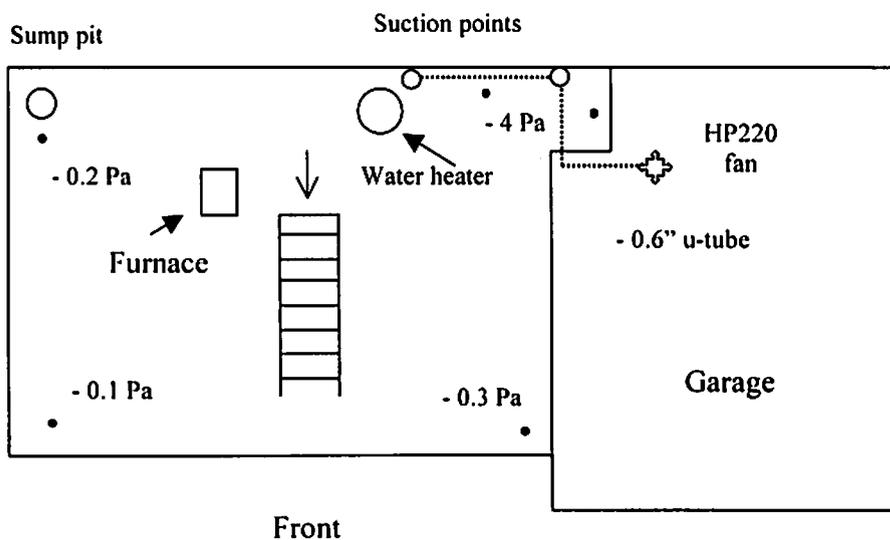
The Office of Surface mining hired another contractor to seal the perimeter canal drain with non-shrink grout and all cracks with a special sealant. Subsequent measurements revealed that the CO<sub>2</sub> levels had decreased but were still present.
