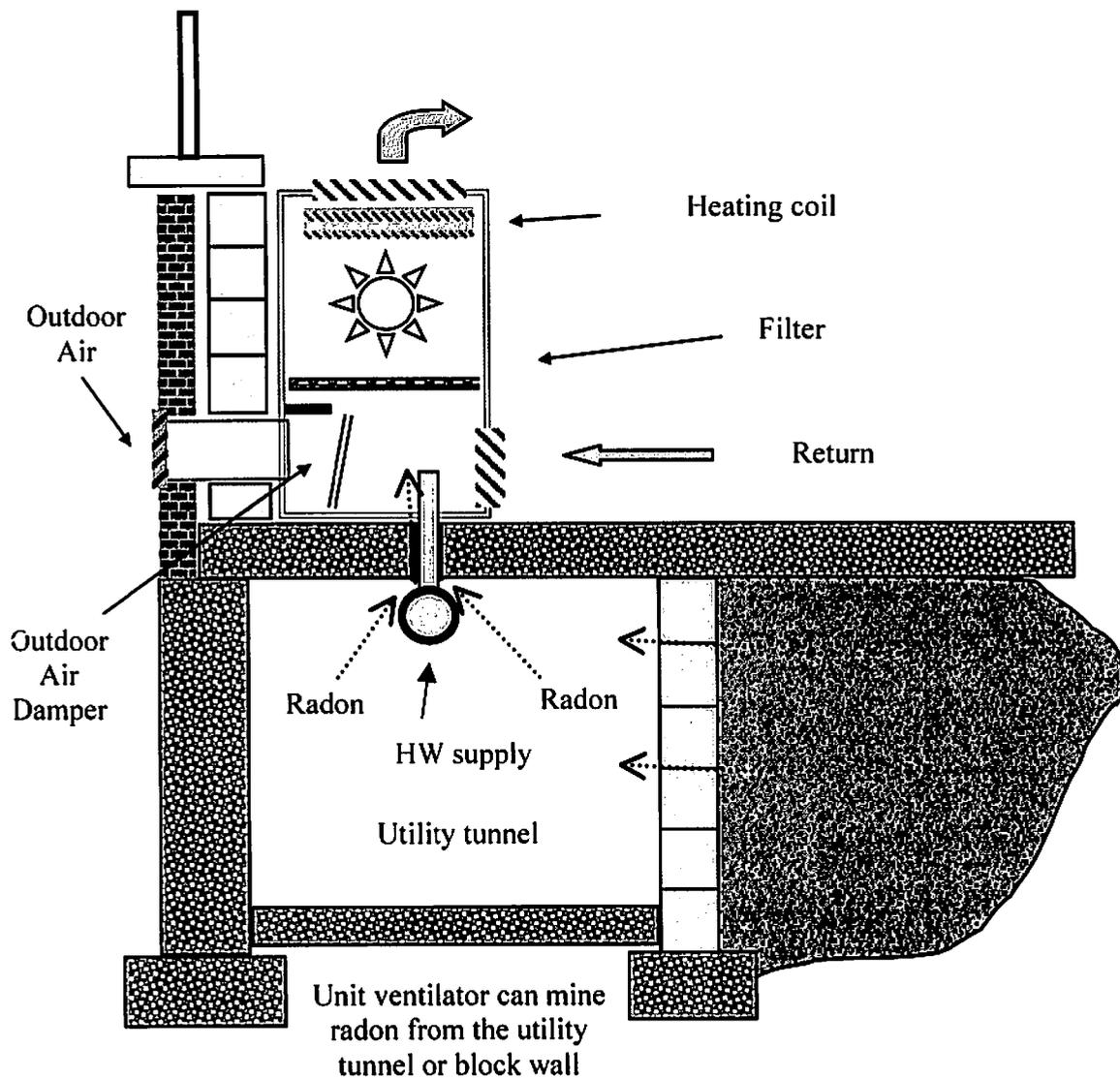
If a school has a central HVAC air handler, it may be mining radon if any of the return ducts are located near radon sources or are depressurizing areas adjacent to the soil. Any return ducts routed through tunnels, crawl spaces or under slabs need to be carefully inspected. Any openings in the bottom half of unit ventilators might be mining radon when the units are running.
