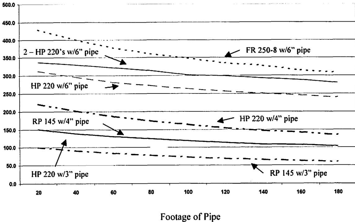
The graph above clearly shows the difference using larger pipe sizes has on airflow. An RP145 uses half as much power as an HP220 fan and yet will move more air in a 4" pipe than a HP220 can move in a three inch pipe.
