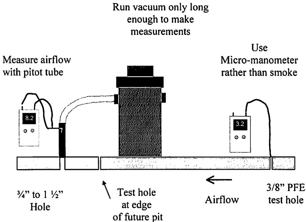
The airflow coming out of the suction hole is measured by placing a 2" pvc pipe over the suction hole and attaching the vacuum hose to the top of the 2" pipe. The velocity pressure in the 2" pipe is measured with a micro-monometer and a pitot tube. The square root of the velocity pressure using inches of water column scale is multiplied times 4000 and then multiplied times the square foot area of the pipe to determine the CFM of air flow.
