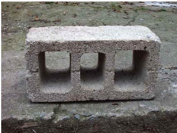
Photo 1 – Hollow Concrete Block
