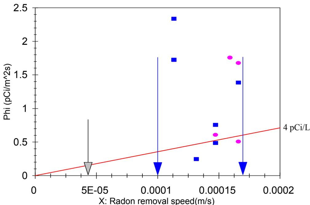
*Fig. 6: Ground Flux (Radon Source) versus Radon Removal Speed (A Building Characteristic). Buildings above the line are predicted to be high after construction if no RRNC is applied.*
