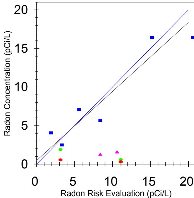
*Fig. 5: Comparison via a correlation diagram for RRE measurements on sites and Radon test values in completed buildings (blue squares). Black line: best linear fit. Circles and triangles: various types of RRNC implemented.*
