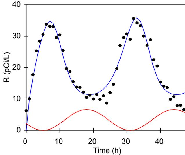
*FIG. 2 Sinusoidal cyclic ventilation function ( $g(t)$ , red curve) allows a good two-parameter fit with data of radon concentrations,  $R_1$ , measured with a CRM detector.*
