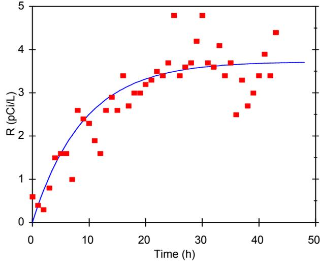
FIG 1: Data from a CRM compared with a numerically evaluated temporal behavior for an increasing radon concentration by radon trapped in a house with  $1/G=T=10$  hours and  $1/\Gamma=\tau=3.825$  days=91.8 hours. Data taken in a house that was in open conditions before  $t=0$  h and closed after  $t=0$  h. Notice that the scatter of data is relatively large. This is because the radon levels are relatively low. (Data taken with femto-Tech CRM-510)
