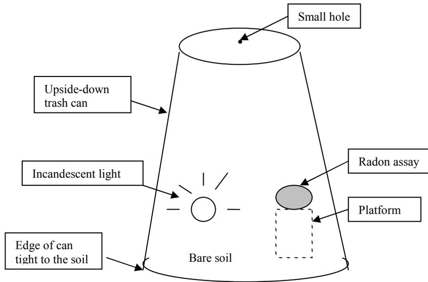
**Figure 1. Schematic of soil-gas-house model, the “Red Box.”**
