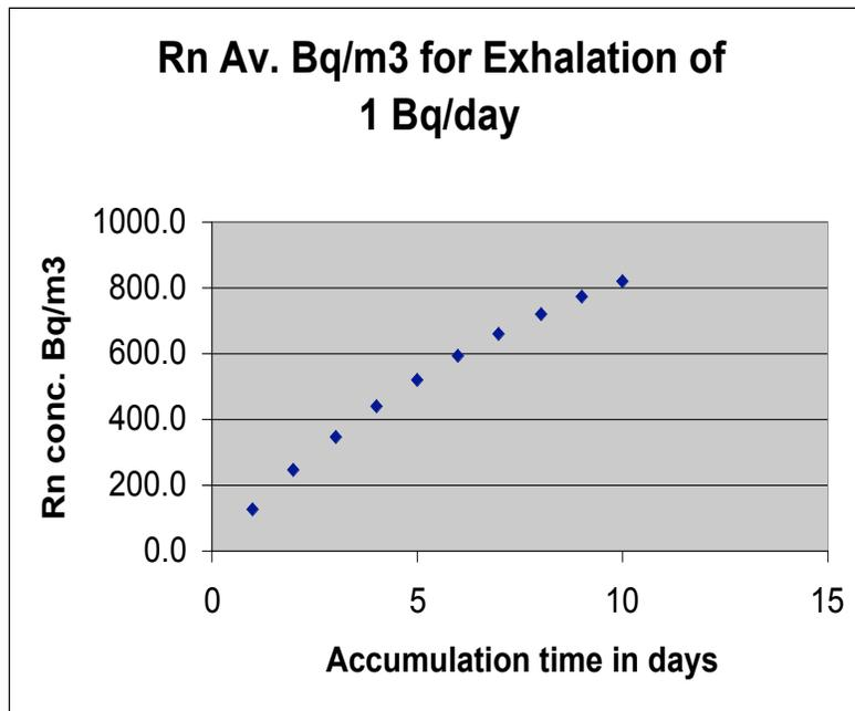
**Figure 2 Build up of time averaged radon concentration for stated accumulation time**
