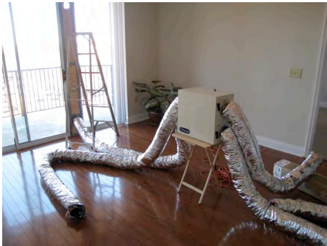
Figure 16 Small ERV being tested for effectiveness
