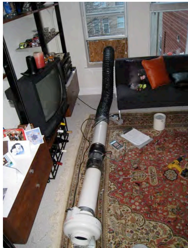
Figure 6 Blower door set up
