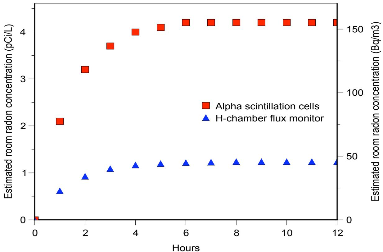
Figure 1. Estimate of radon ingrowth in a 20 m<sup>3</sup> room from granite countertop material based on measurements conducted using a H-chamber flux monitor and alpha-scintillation cells.
