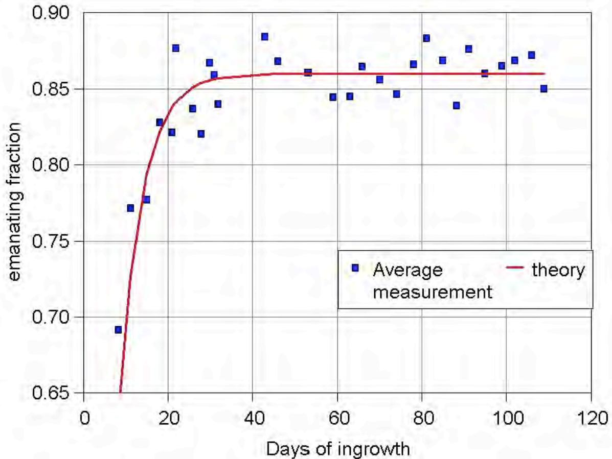
Fig. 1. Decay-corrected activities in the cocktails indicate that secular equilibrium is established within 40 d.
