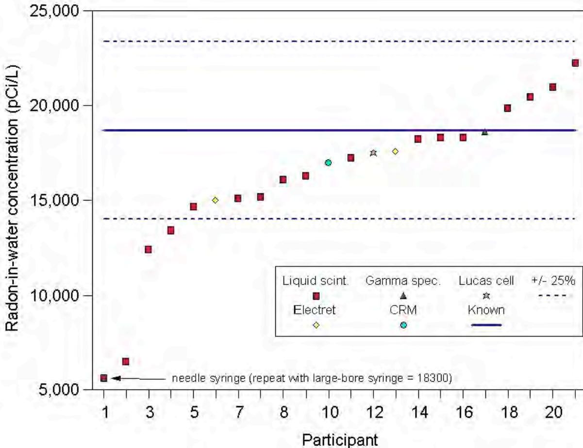
Fig. 2. Results of a radon-in-water intercomparison conducted in 2008 show that 18 of 21 participants reported concentrations within 25% of the known value (18,700 pCi/L).
