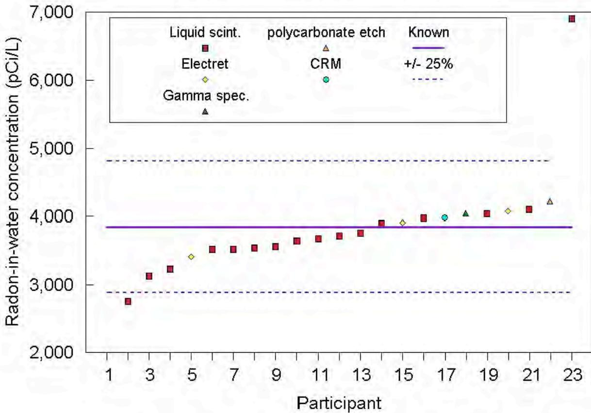
Fig. 3. Results of a 2009 radon-in-water intercomparison conducted in 2009 show that 21 of 23 participants reported concentrations within 25% of the known value (3850 pCi/L).
