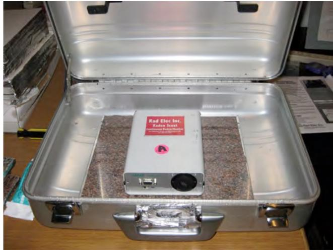
Fig 5 Enclosure accumulator with CRM and granite sample
