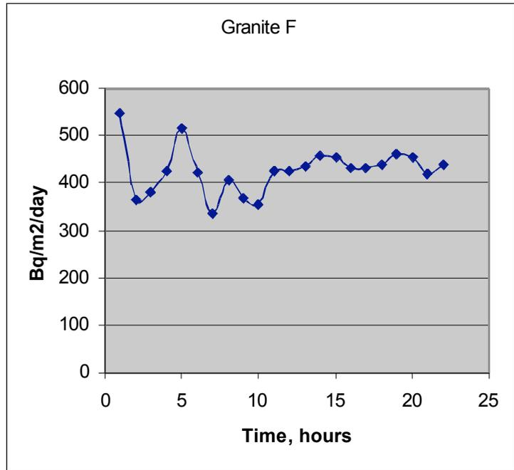
Fig 4 Calculated Radon Flux at stated accumulation time
