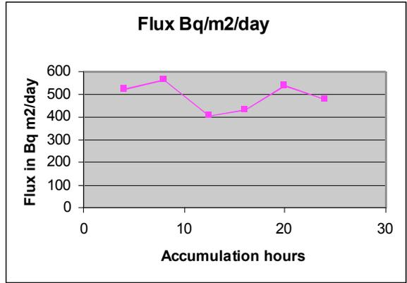
Fig 3 Calculated Radon Flux at stated accumulation time
