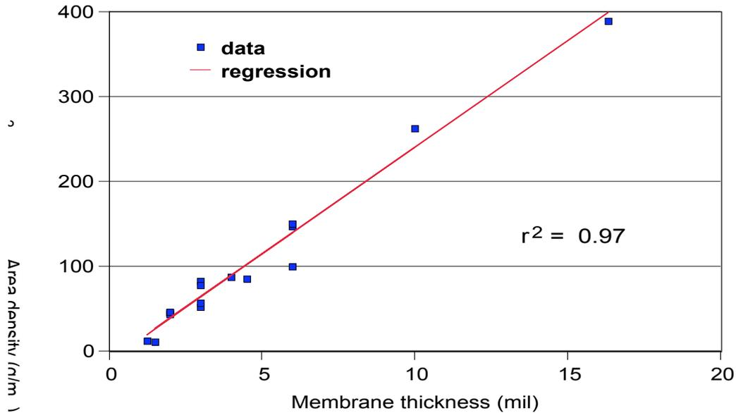
Fig. 1. Membrane thickness is strongly correlated with area density for the materials studied. Table 1. Description of membranes tested.
