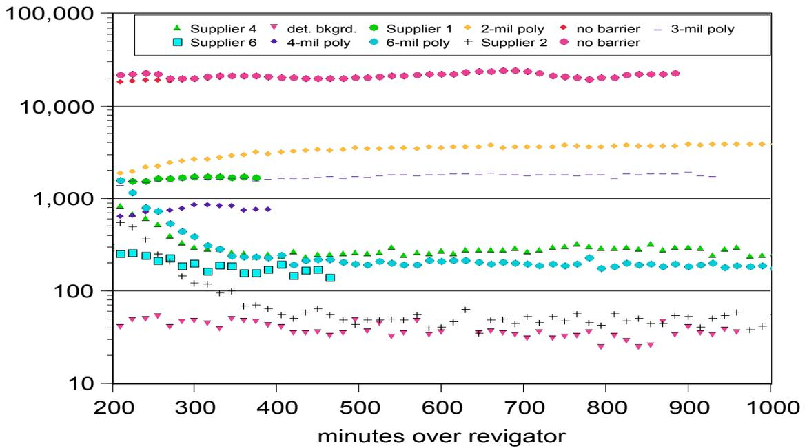
Fig. 3. Count rates measured with membranes separating continuous radon monitor and revigator (initial setup 2A).
