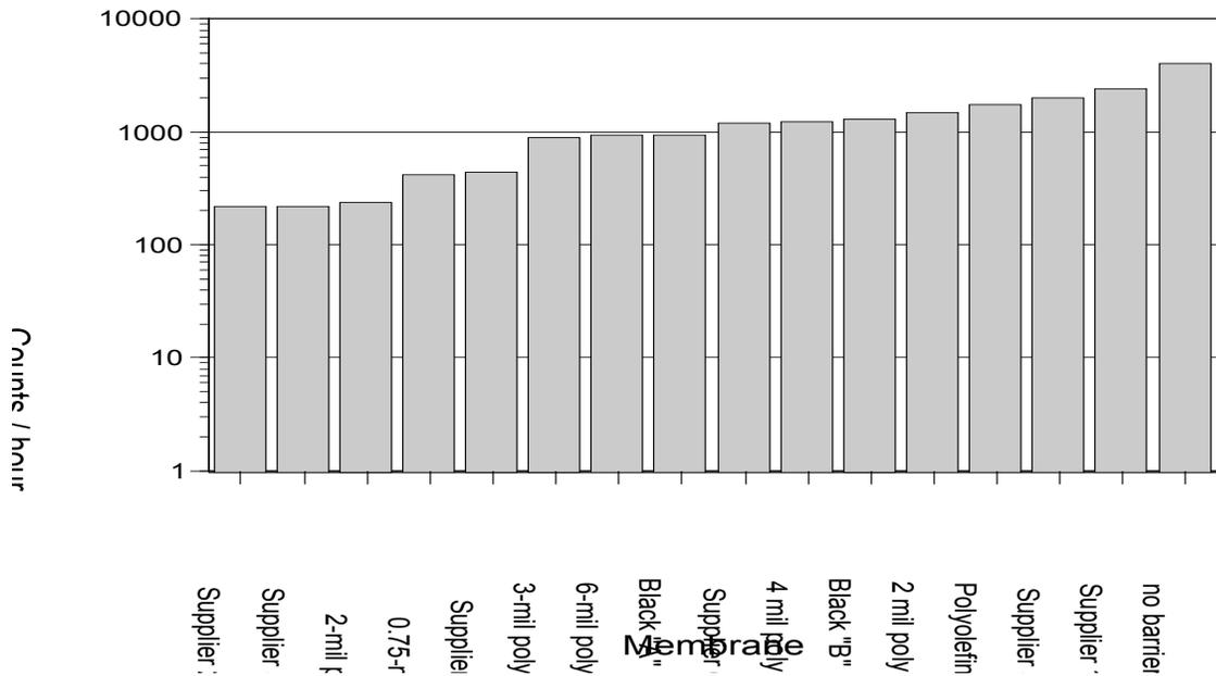
Fig. 6. Count rates measured with membrane separating continuous radon monitor and <sup>226</sup>Ra capsule inside airtight chamber (setup 2C).
