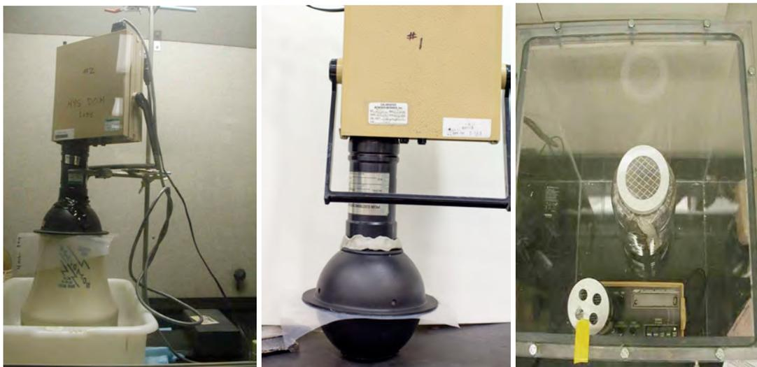
Fig. 2. Experimental setups that were used to examine the permeability of membrane materials: continuous radon monitor mounted over water-filled Revigator (A);  $^{226}\text{Ra}$  capsule and continuous radon monitor (B); and covered glass jar containing  $^{226}\text{Ra}$  capsule in airtight chamber (C).
