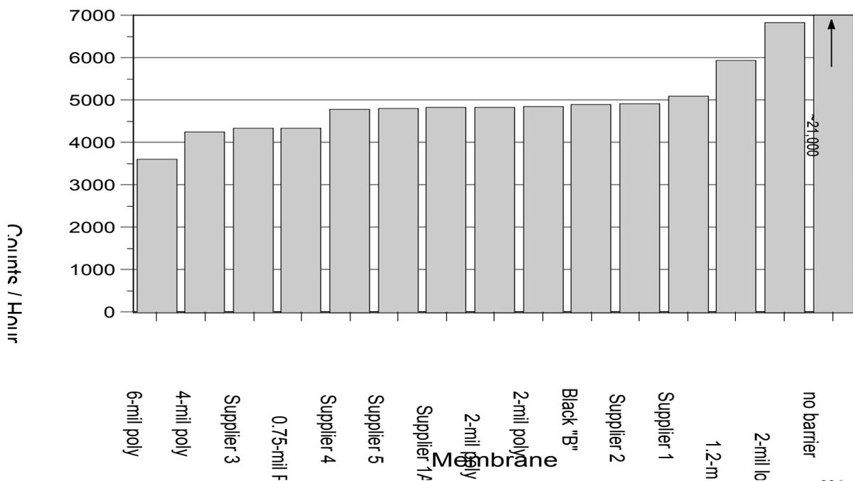
Fig. 5. Count rates measured with membranes separating continuous radon monitor and  $^{226}\text{Ra}$  capsule (setup 2B).
