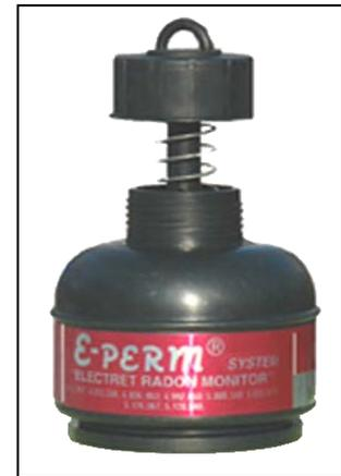
Figure 4. Rad Elec electret ion chamber
