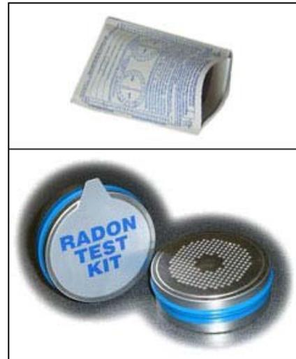
**Figure 2. Airchek (top); RTCA charcoal canister (bottom)**
