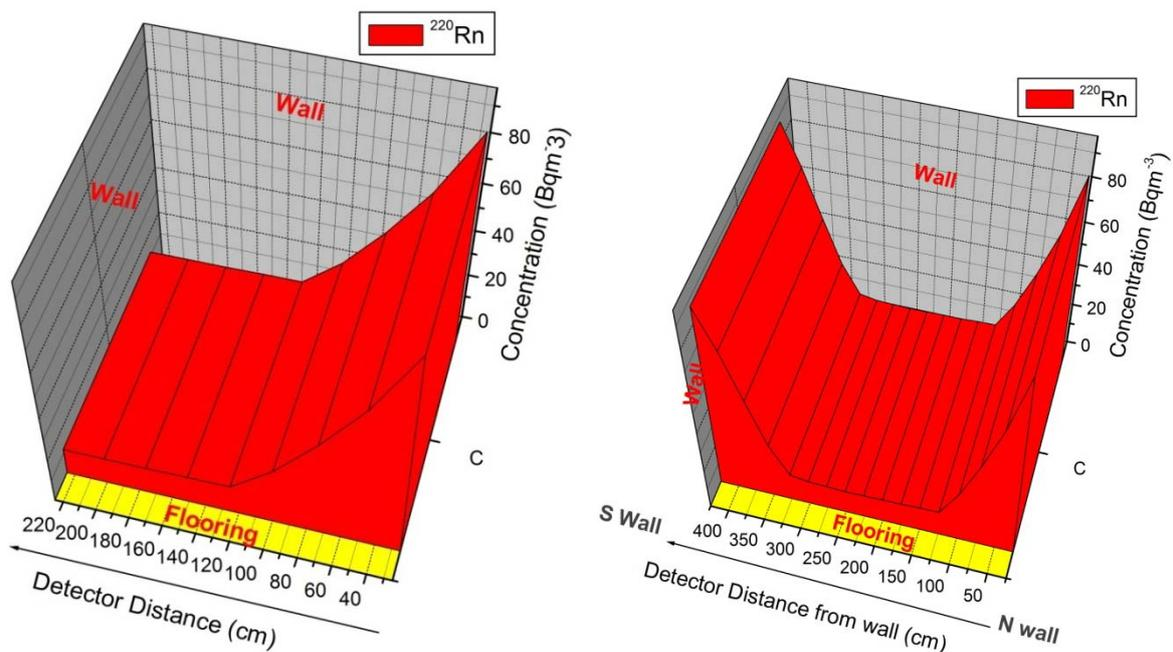
Fig.5: Horizontal distribution of <sup>220</sup>Rn in a dwelling Fig. 6: Distribution of <sup>220</sup>Rn concentration from the wall
