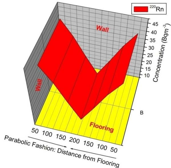
Fig. 10:  $^{220}\text{Rn}$  level when the dosimeters placed in upper parabolic fashion: Distance from flooring
