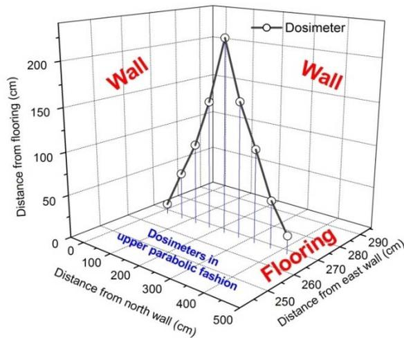
Fig.4: Deployment of dosimeter in upper parabolic fashion
