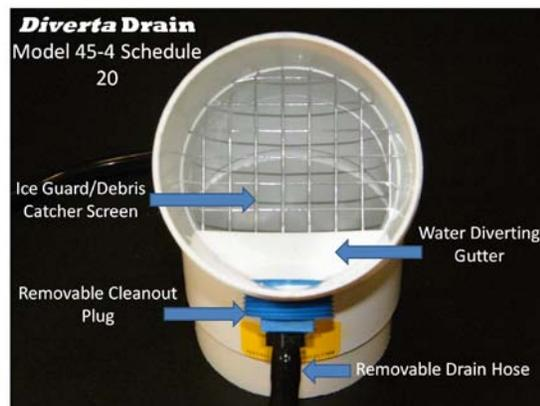
Figure 2 – Features of Diverta Drain
