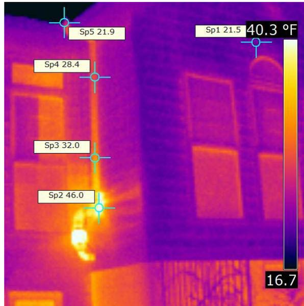
Figure 1 – Thermal Image (Temperature differences within radon system piping).
