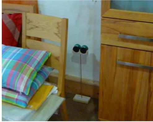
Figure (2): Placement of a combined radon and thoron and a thoron-only passive measurement device at a distance of 20 cm from a clay paneled and rendered wall.
