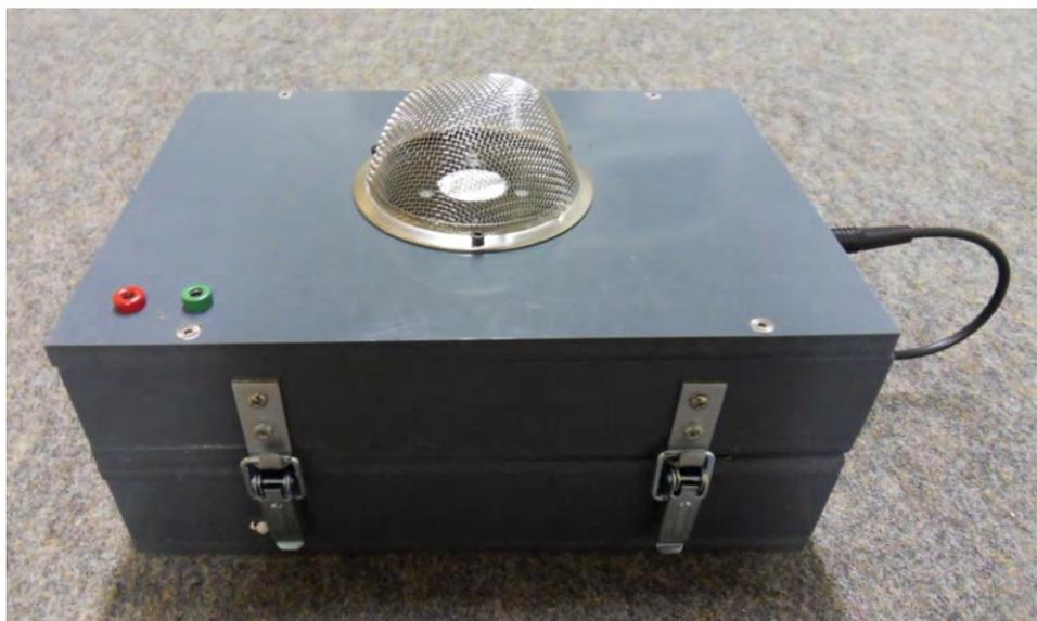
Figure 1: Photo of one of the passive UBPM thoron progeny measurements devices used in this study.
