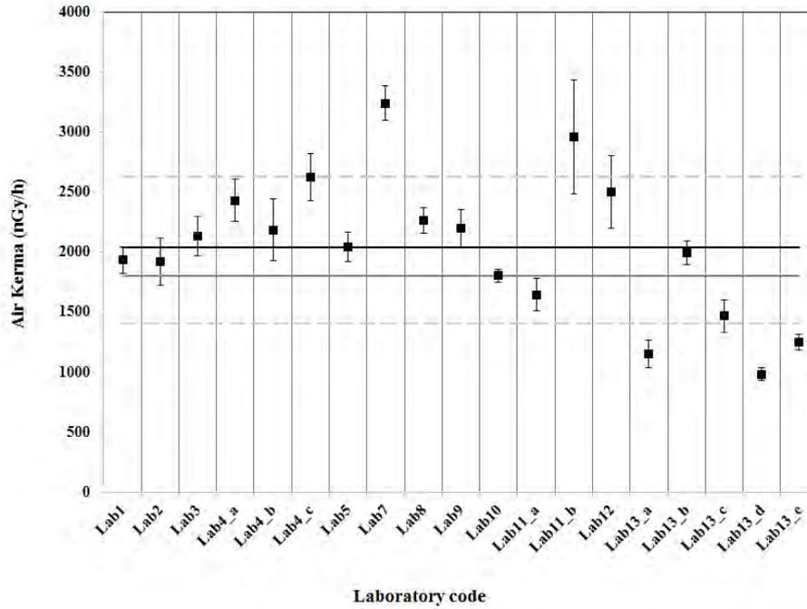
Figure (6): Results of the test in the reference point with high levels of external gamma dose
