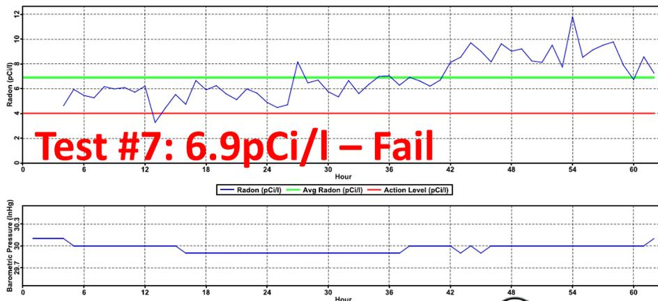
Figure (3): Graphics provided by Radalink for Test #7 showing a failing score of 6.9 pCi/l
