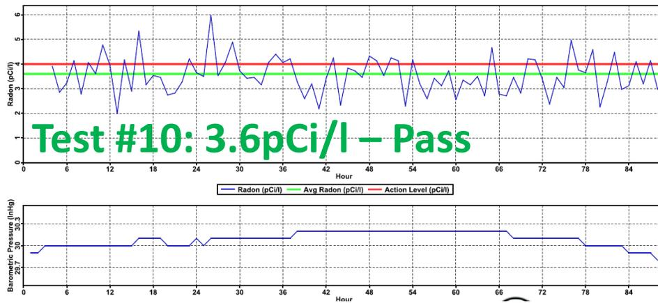
Figure (2): Graphics provided by Radalink for Test #10 showing a passing score of 3.6 pCi/l
