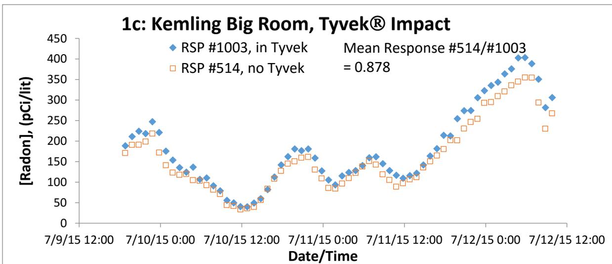
Figure (1): Impact of Tyvek barrier bags and orientation on RSP radon measurements.
