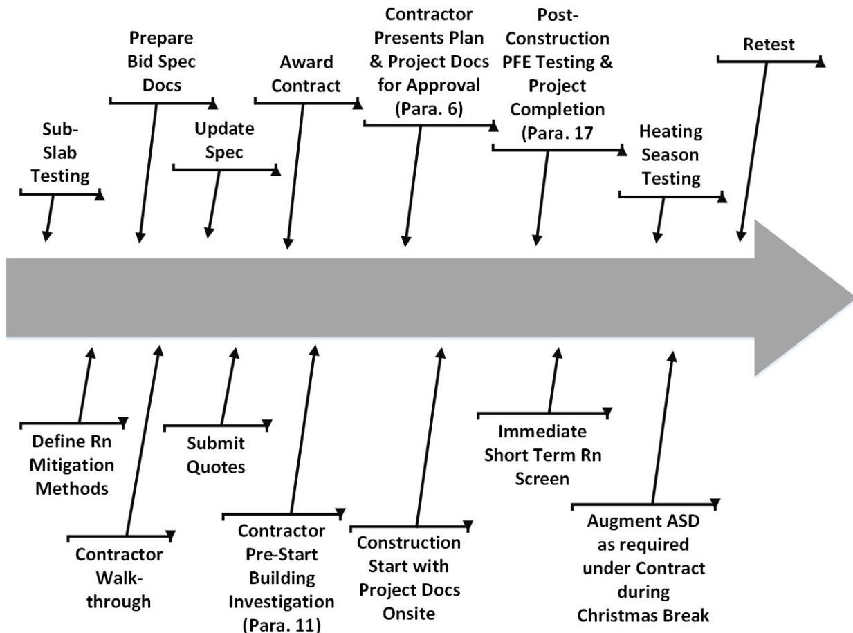
Figure (1): Radon mitigation project timeline <sup>1</sup>
