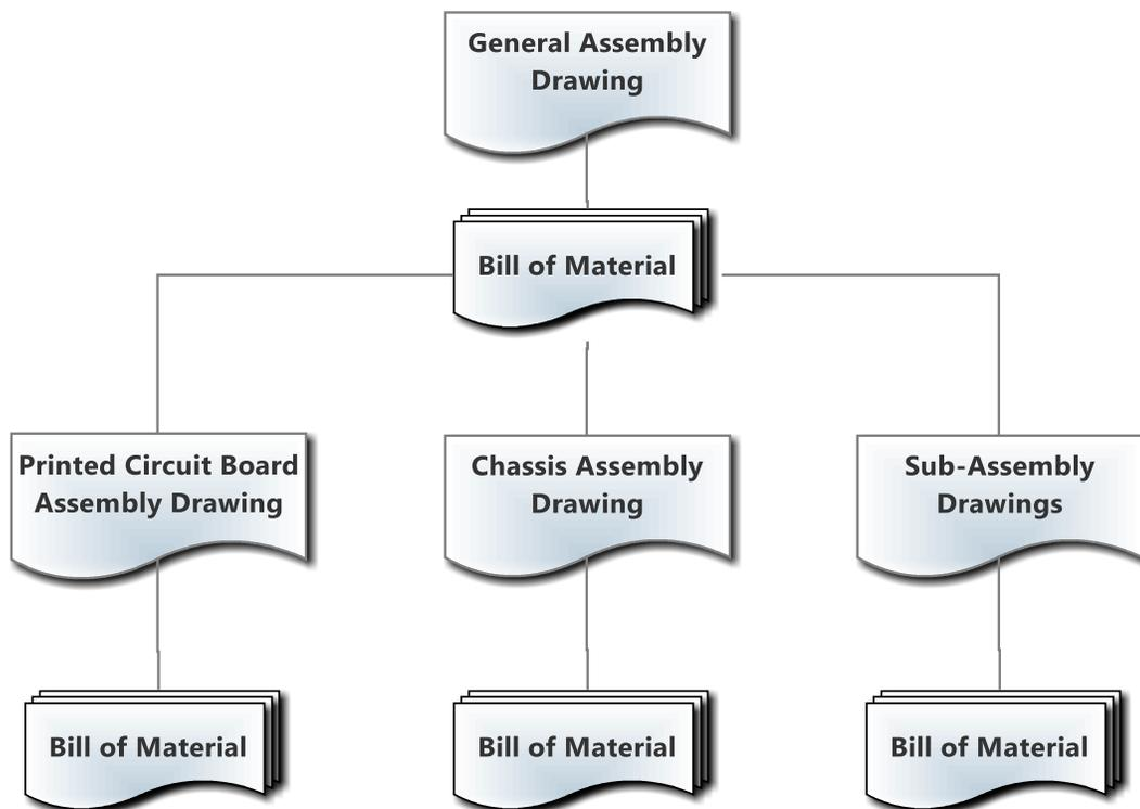
Figure (3): Typical CRM or EID General Assembly Drawing and Bills of Material Relationship
