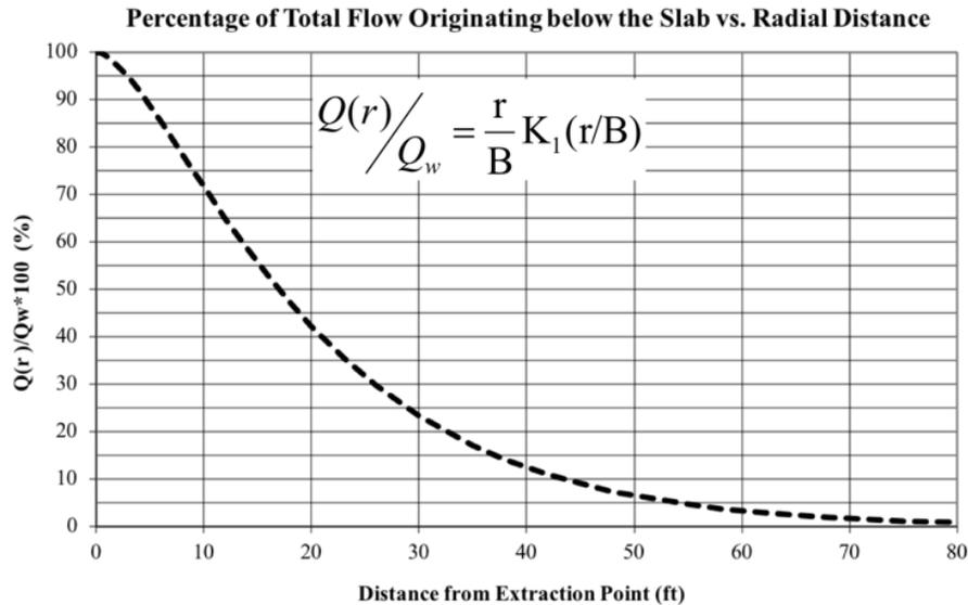
Figure (5): Proportion of flow originating below the floor vs radial distance
