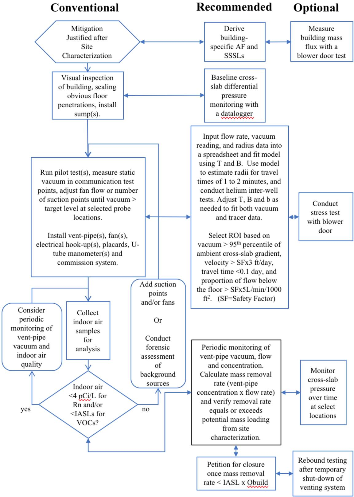
Figure (6): Logic flow diagram for mitigation system design and performance monitoring.
