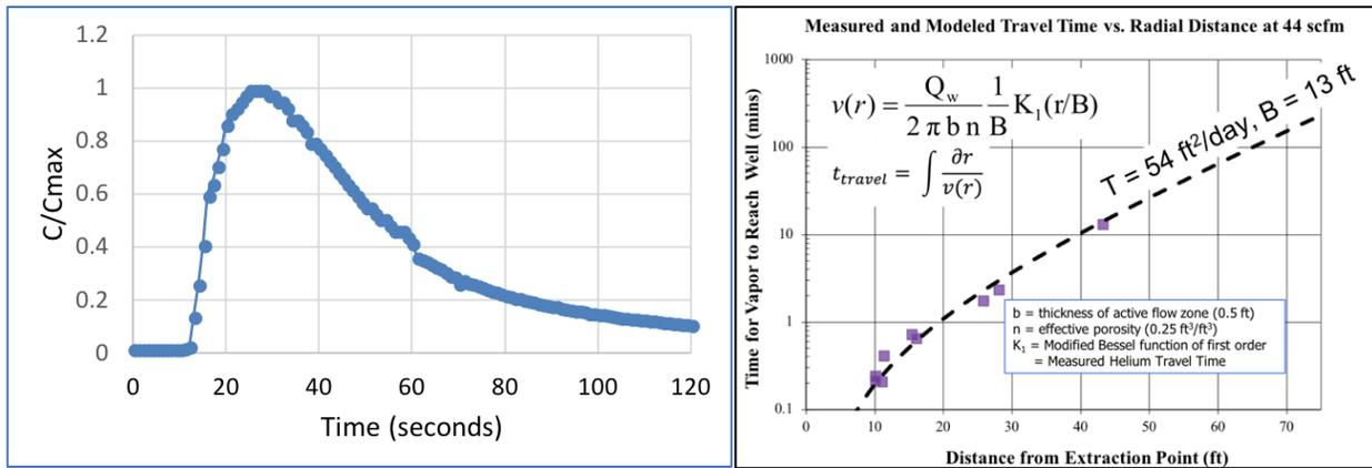
Figure (4): Measured (left) and modelled (right) travel time vs distance from suction point
