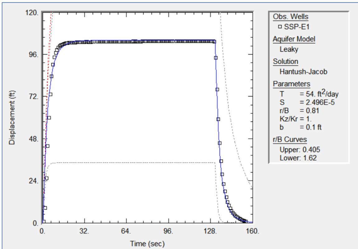
Figure (2): Example of subslab vacuum vs time: raw data (top), and fit to the Hantush-Jacob Model (bottom), using AQTESOLV, by HydroSOLVE, Inc. of Reston, VA
