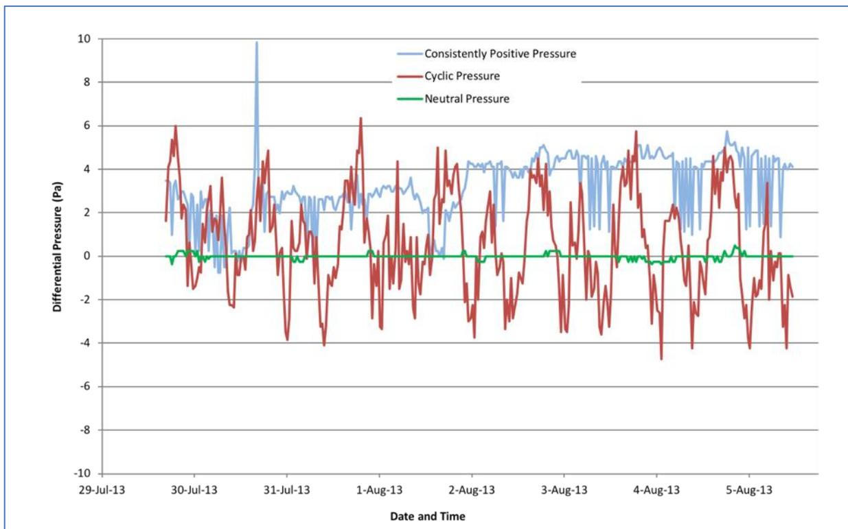
Figure (1): Example of cross-slab differential pressure for three buildings with no SSV systems
