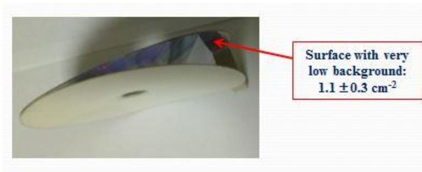
Figure (1): The structure of a DVD: it consists of two halves stuck together. The front half is made of polycarbonate which can be used as alpha-track detector. The background of the internal polycarbonate surface is very low, and can be additionally reduced by thermal annealing.
