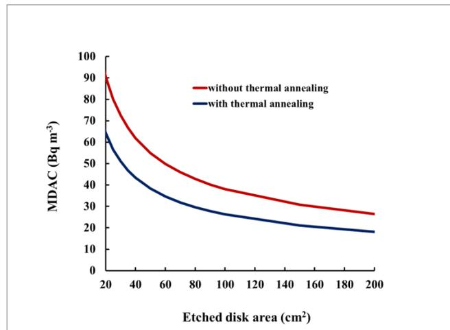
Figure (6): Minimum detectable average <sup>222</sup>Rn concentrations after one week of exposure of “packed detectors” as dependent on the surface which is etched and tracks are counted.
