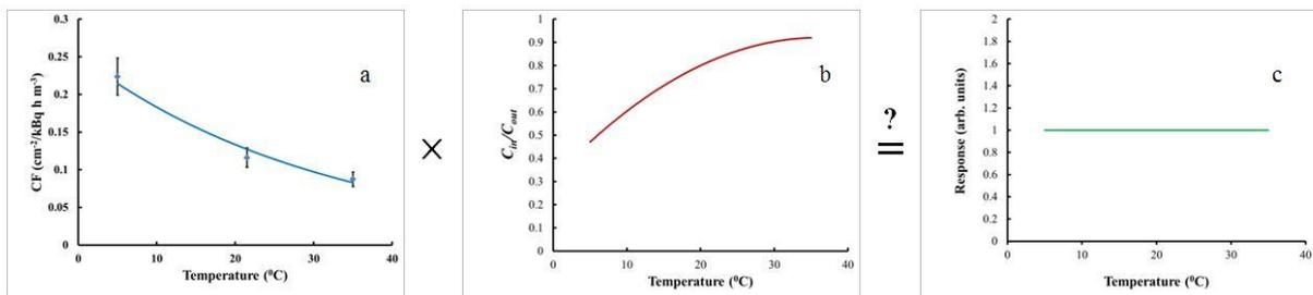
Figure (3): (a) Temperature dependence of the  $CF$  of detectors; (b) Typical dependence on the temperature of the ratio  $C_{in}/C_{out}$  in a volume in which radon penetrates by diffusion through plastic wall(s) (Tommasino, 2016); (c) The concept: would it be possible by placing the detectors (a) in a volume (b) to achieve compensated temperature dependence of the response.
