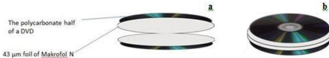
Figure (2): (a) Scheme of the detector element; (b) Detector element ready to use.
