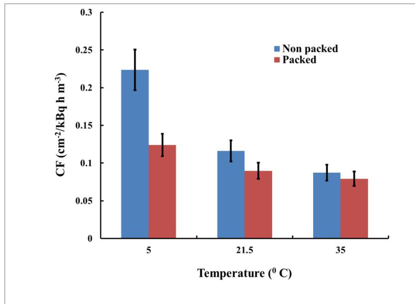
Figure (5): Dependence of the CF on the temperature of packed and not-packed detectors. The temperature dependence of packed detectors is significantly reduced.
