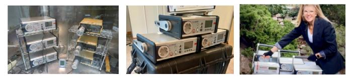
environment. For these final exposures, a fourth AlphaGUARD loaned by the US EPA Las Vegas laboratory joined the lineup. The four instruments were exposed to outdoor concentrations as low as a tenth of a pCi/L and indoor concentrations as high as 150 pCi/L as part of their final assessment.
